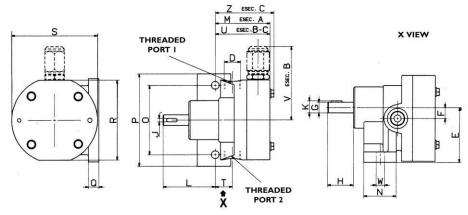
Max Pressure = 30 bar for continuous working − Max Pressure = 60 bar for intermittent working. Fluid working temperature = 20÷100 °C with low and medium oil viscosity.
