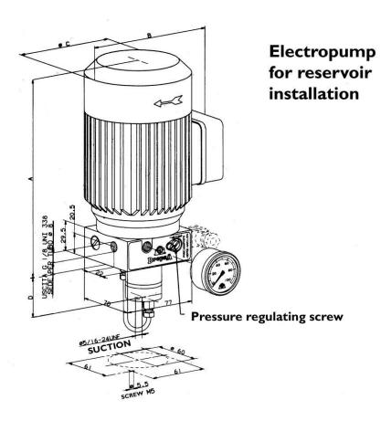
This assembly consists only of the motor and the gear pump.
