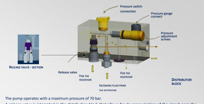
A release valve is integrated in the distribution block that allows for de-pressurisation of the circuit once the lubrication cycle has ended.
