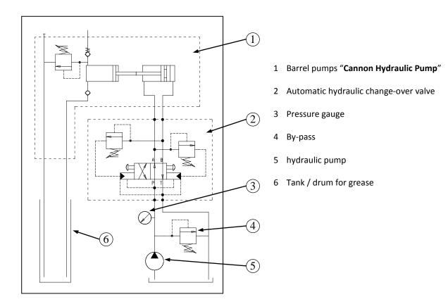
**HydMin Pump** is suited to automatic lubrication system for mobile and fixed systems where no electrical power is present. Typical such applications require that grease is pumped at pressure (for example bearings, hubs, studs, joints, etc..) in quarries, mines, industrial and manufacturing applications.
