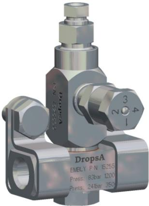
These injectors have a visual indication pin incorporated within the valve to confirm proper lubrication. The valves are mounted on manifolds available from 1 to 7 outlets.
