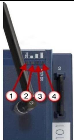
Note: If all signal level LEDs are off, there is no signal.
